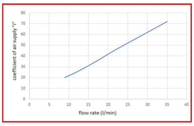
air flow rate (NL/min) = i \* inlet working pressure (bar)
