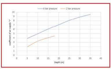
Variation in the pump flow rate according to the operation depth.
