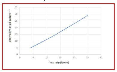
air flow rate (NL/min) = i \* inlet working pressure (bar)
