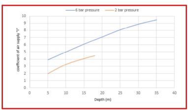
Variation in the pump flow rate according to the operation depth. This graph is referred to 2 m hydrostatic head and 6 bar pressure of compressed air supply
